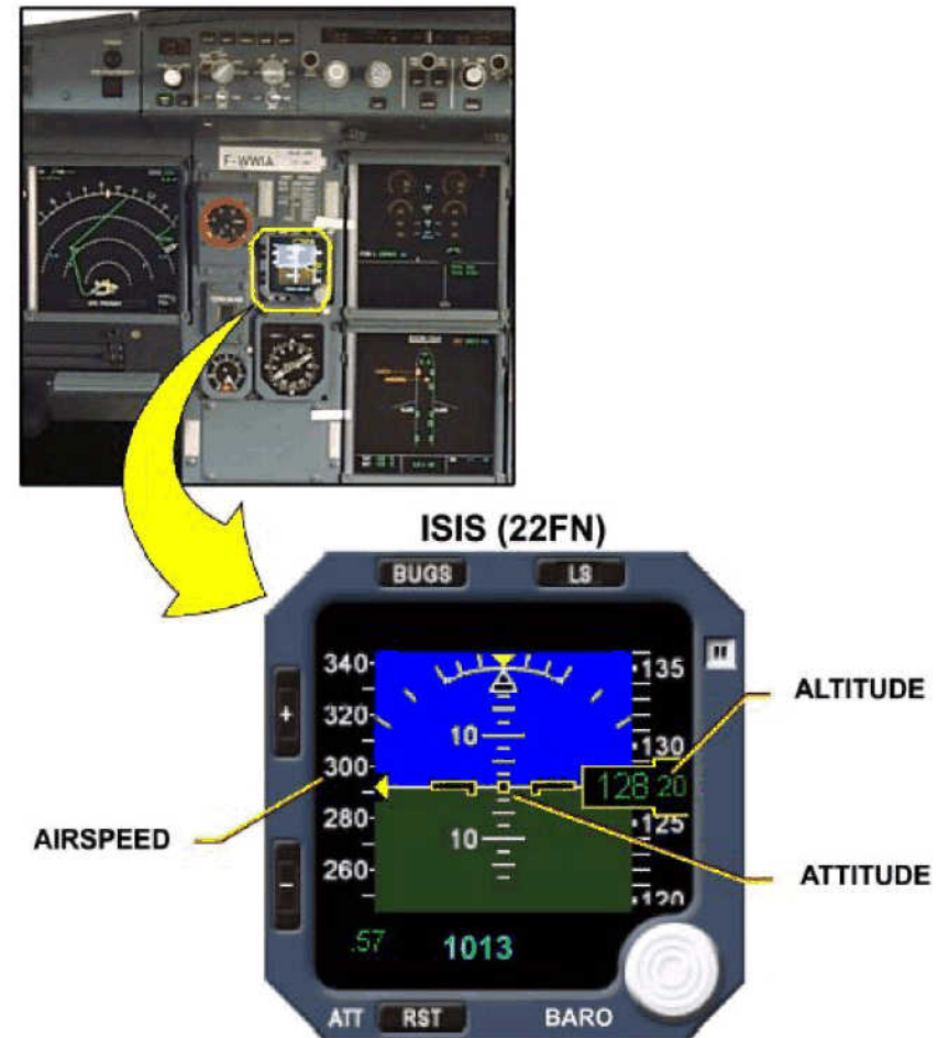
Figure 53 Standby Instrument Panel
